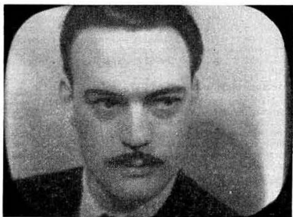
An unretouched photograph of the results seen on the monitor screen of G3AST (Luton). The original was a photographic negative, the scanner a 5FP7 and the monitor a VCR97. The picture shows the excellent results obtainable with simple equipment.
